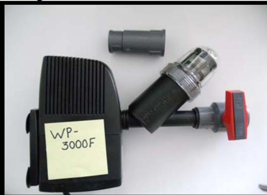
Your replacement pump can now be plugged in and started. You may also have to prime your pump by unplugging it, waiting 5 seconds, plugging it back in, and then repeating. Please also note that the red and grey handle in the pictures is the water flow control valve. The flow control valve in all of the pictures is closed. By turning the opposite way you would completely open the valve.
